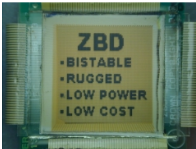
Figure 8: Reflective twisted unpowered ZBD display. Grating made in S1813.
